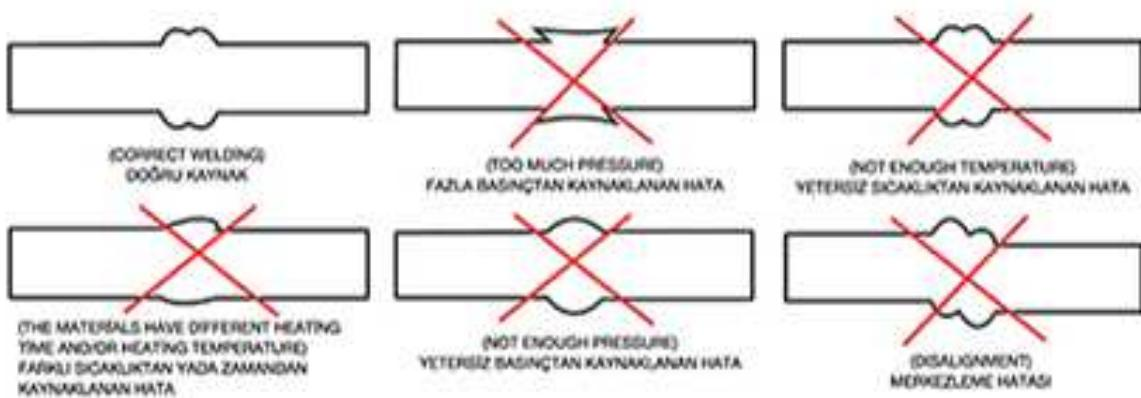
**IMPORTANT: PULLING PRESSURE + PRESSURE ON DIAGRAM + WHILE ON WELDING PROCESS.**
